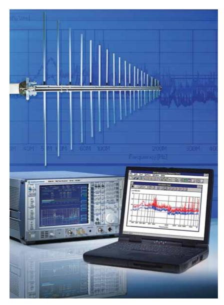
Fully automatic operation supported by the Rohde&Schwarz EMI test receivers and a large number of accessories such as mast, turntable, absorbing clamp/ slideway and artificial mains networks make even complex EMI measurements reliable and fast over a wide frequency range. The interactive mode lets operators utilize their experience to the full and identify and catalog signals in open-field measurements, for example.
